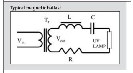
the power in kW. The most common power source is the 120-volt, 15-amp residential outlet delivering a maximum of 1.8 kW. Other outlets deliver 220 volts at 15, 20, 30 and 50 amps delivering 3.3 kW, 4.4kW, 6.6 kW and 11 kW, respectively. Typical UV lamps operating at these power levels require magnetic ballasts weighing 62, 80, 93, 120 and 172 pounds, respectively. The entire system, however, can weigh more.
