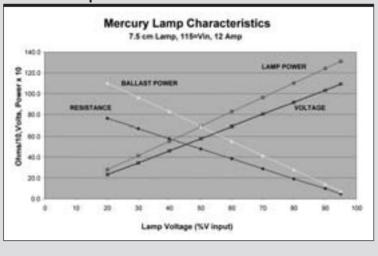
Figure 6 illustrates the lamp's characteristics with a constant 12-amp current level. For this example, the resistance of the ballast is decreased linearly by electronic means.
