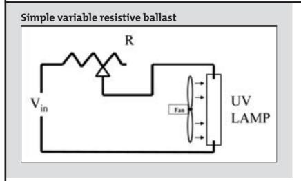
voltage can now be tuned by adjusting gas-cooling parameters and resistance.
